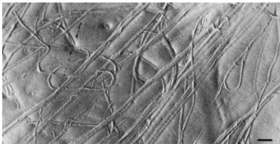
Figure 4. Freeze-fracture electron micrograph showing molecular aggregation of compound 2 into linear and helical fibers and macrofiber bundles in dichloromethane (scale bar represents 200 nm).
